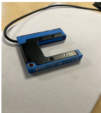
(Ticket machine sensor)
